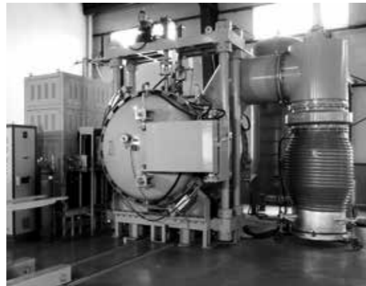
Vacuum oven for PACOPLATE production, in which various cloth layers are repeatedly laminated to produce high quality composite materials. The final product is extremely efficient, easy to form and corrosion resistant. All functional characteristics such as pore size, distribution and flow characteristics are exactly and permanently fixed.
