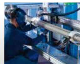
PACO employs welding systems designed and built by the in-house mechanical engineering team for the production of its filters – for example, to produce extremely long filter elements (up to 4.200 mm).
