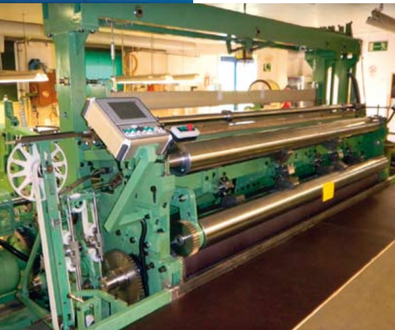
The new PACO HD "Wide Loom" 3000 Built in the PACO factory in Herolz and already working reliably and failure-free for six months to produce precision metal cloths of various specifications.
