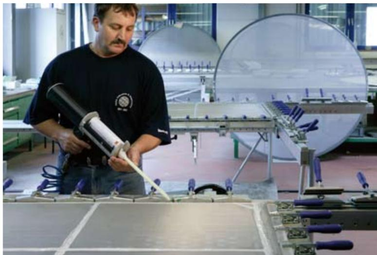
The qualitative harmony between sieve cloth, frame and screening is an important feature of PACO screens for the fibreboard industry.
