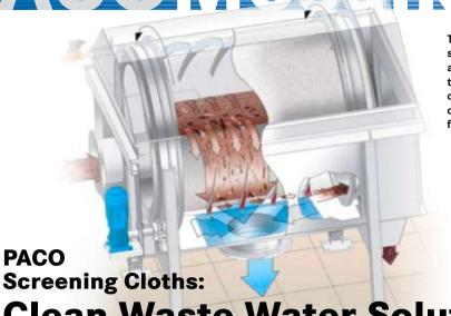
The combination of fine screening with simple cleaning and forced separation enables the RoMesh® System to continuously and safely separate large concentrations of fine solids from waste water.
