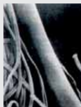
Difference in size between a yarn consisting of many microfibres (left) and a human hair (right).
