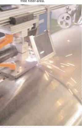
Unit for plasma-cutting PACO-Autoscreen-mesh preventing from unravelling in the later processes.
