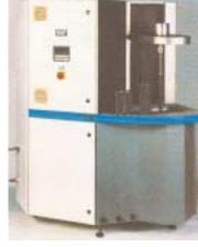
"Clean it, don't trash it" is the motto of the "Two-mode" ultrasonic cleaner with hot fluid flushing made by Bodensohn Präzision, Seligenstadt, Germany. After just three minutes of cleaning, a PACO metal filter from a diesel engine is 100% fit for re-use.
